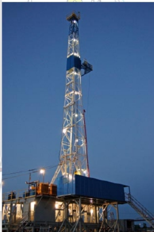
Drilling Rig: IDECO 725 Rig Type: Trailer Mounted Drilling and WorkOver Rig
